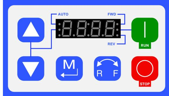
Figure 7 VFD Control Panel
