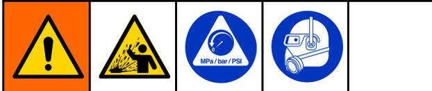
This equipment stays pressurized until pressure is relieved manually. To help prevent serious injury from pressurized fluid, such as splashing in the eyes or on skin, follow the Pressure Relief Procedure when you stop pumping and before you clean, check, or service the equipment.
